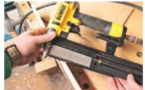
Nails are easy to load; the yellow tab to the right of the nail track indicates if the gun is empty
